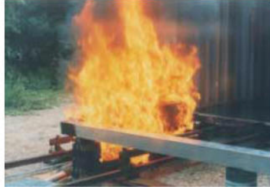
30-min fire test on a ZEBRA battery
